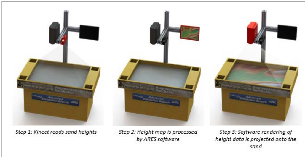
Fig. 2 Terrain recognition process
